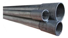
Heavy protection welded steel electrical conduit, screwed both ends with one end complete with plain coupling. Hot dipped galvanised steel conduit is used in applications where mechanical strength is required in corrosive environments or to conform to specific requirements.
