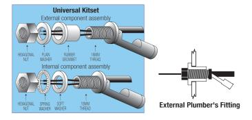
Note: Suitable for control/signalling only. Refer to wattage.
