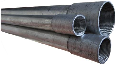
Heavy protection welded steel electrical conduit, screwed both ends with one end complete with plain coupling. Hot dipped galvanised steel conduit is used in applications where mechanical strength is required in corrosive environments or to conform to specific requirements.
